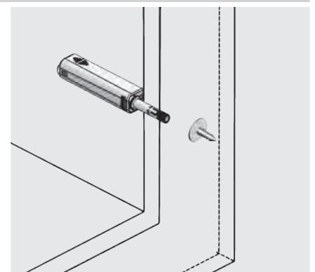
**Push-Open Adjustable Adapter of Inside Cabinet "For Long Latch"**
