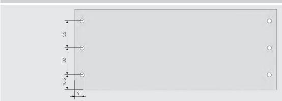
\* All dimensions in the diagram are in mm.
